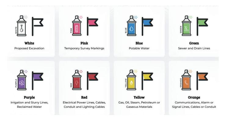
Within the City of Woodway, our Public Utilities crews will be notified by 811 to mark the main water or sewer lines (BLUE or GREEN). However, as the lines from your house to the water and sewer mains were installed on private property by plumbing contractors, City staff are unable to locate and mark these lines. We are also unable to mark private irrigation lines. These are typically located, when necessary, by a plumbing or irrigation contractor.
